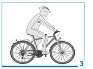
When one pedal is forward, the knee is over the axle of the front pedal (see "Illustr.: Optimum seating position (3)").
