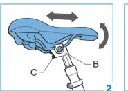
Never pull up the saddle pin higher than the marking on the saddle pin, see page 9.
