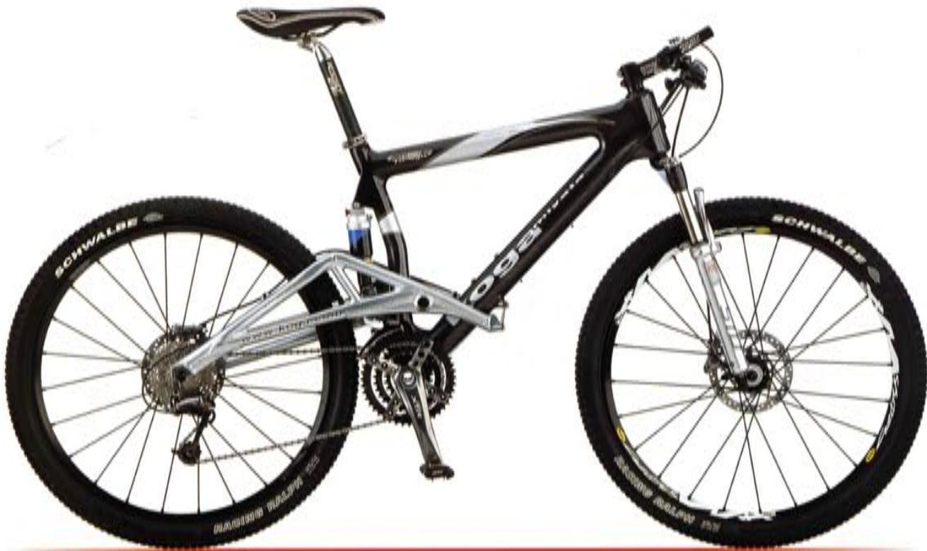
**X-ControlCarbon (XCC)** Framematen 41-46-50-54cm **Framemateriaal** Carbon **Voorvork** Rockshox Sid Worldcup, travel 80mm **Kleurencombinatie** Carbon woven/Platinum silver metallic/Smoke metallic **Groep** Shimano XTR incl. schijfremmen **Wielset** Mavic Crossmax XL Disc **Banden** Schwalbe Racing Ralph Evolution 54-599 **Zadel** Selle San Marco Bontrager RaceLine gel **Zadelpen** Ritchey WCS Mtn ø31,8x350mm **Pedalen** Time Atac X3 Carbon **Detailinformatie pagina 81**
